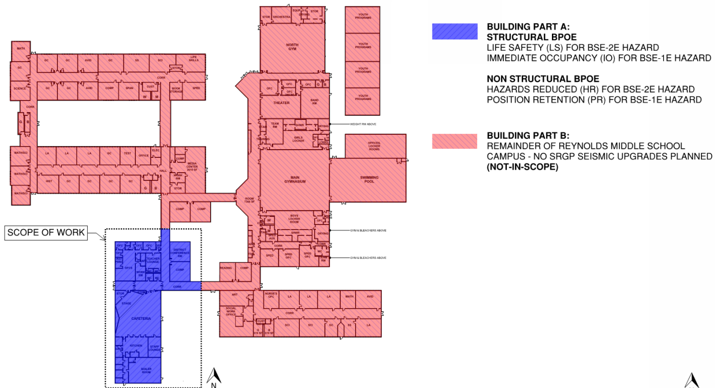
Figure 19: Basic Performance Objective for Existing Buildings (BPOE)
